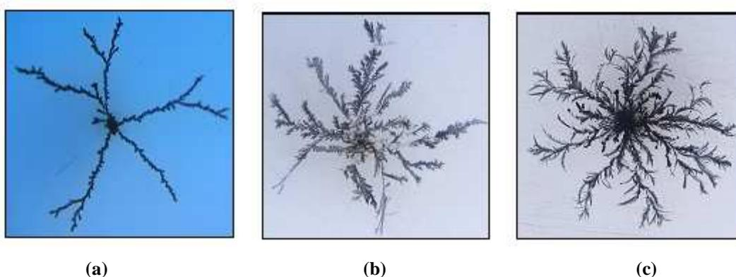
**Figure 1: Original Images of 0.5 Molar a) Copper Sulphate ( $\text{CuSO}_4$ ) b) Lead Acetate  $\text{Pb}(\text{C}_2\text{H}_3\text{O}_2)_2$  c) Zinc Acetate  $\text{Zn}(\text{O}_2\text{CCH}_3)_2$  Under Cell Applied Voltage 7V**
