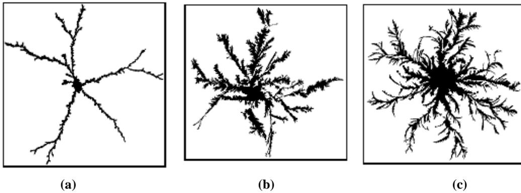
**Figure 2: Two Color Bit Images of 0.5 Molar a) Copper Sulphate (CuSo<sub>4</sub>) b) Lead Acetate Pb (C<sub>2</sub>H<sub>3</sub>O<sub>2</sub>)<sub>2</sub> c) Zinc Acetate Zn (O<sub>2</sub>CCH<sub>3</sub>)<sub>2</sub> under Cell Applied Voltage 7V**
